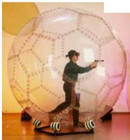
A virtual reality unit that allows the user to move freely in any direction. Photo courtesy of VIRTUSPHERE
